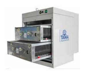
**OPERATING PRINCIPLE — Electrostatic version**The aspired air is routed into the drops separator, that condenses liquid and oily substances. The second stage is formed by a metallic pre-filter that hold the particles with bigger granulometry. Then the prefiltered air passes through the electrostatic cell, where the smallest pollutant are subsided.
