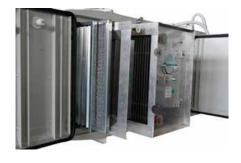
**OPERATING PRINCIPLE — Electrostatic version**The aspired air is routed into the drops separator, that condenses liquid and oily substances. The second stage is formed by a metallic pre-filter that hold the particles with bigger granulometry. Then the pre-filtered air passes through the electrostatic cell, where the smallest pollutant are subsided.
